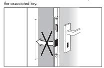
Locking elements must not be misused to hold the door open.
